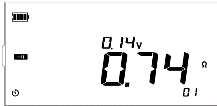
Figure 13.16 Test leads are shorted
